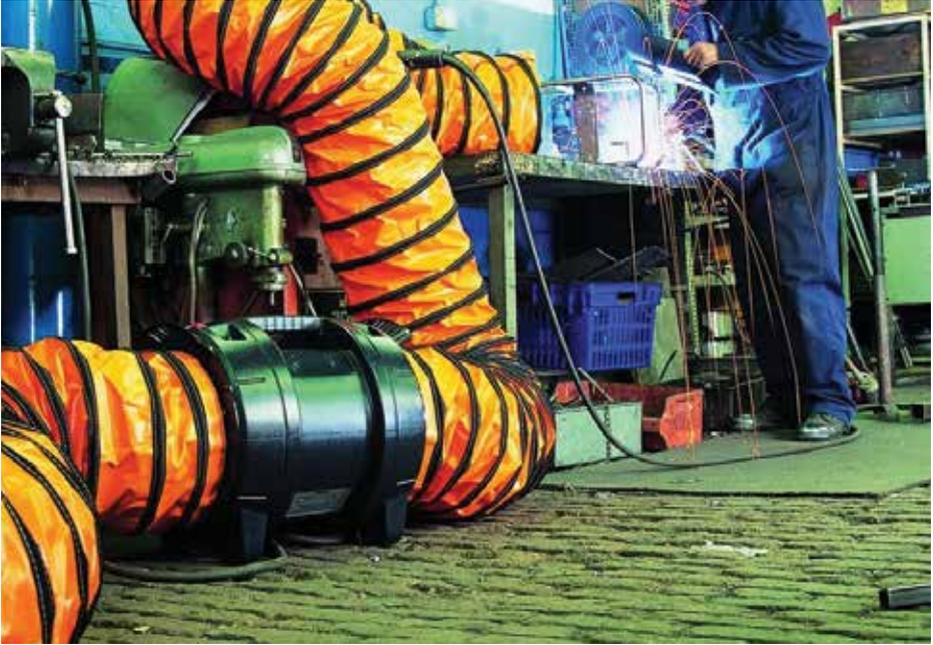
300mm fume extractors c/w 5m duct, 110V. Additional lengths of ducting can be supplied
