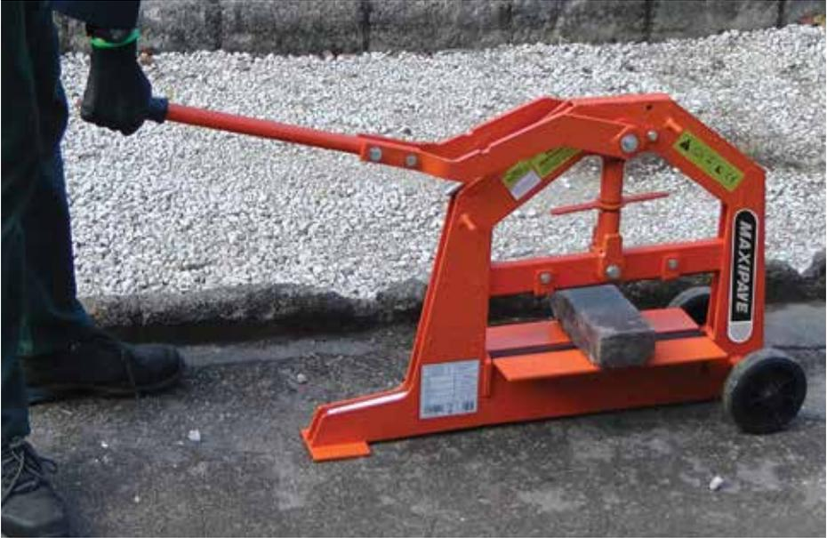
Small paving block cutter
